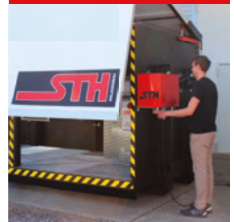
Hydraulic unit for opening the H12
