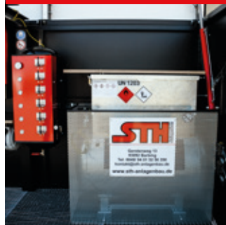
Petrol tank KC500/ operating unit of the pumps
